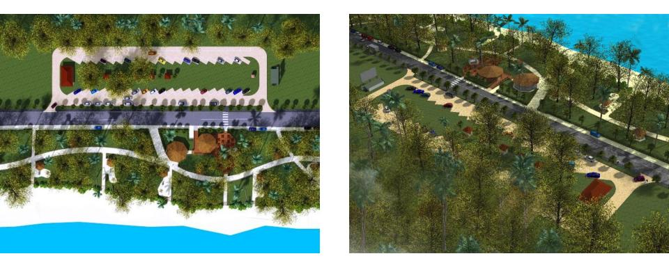
The proposed car park will located on the opposite side of the main road as there is sufficient space and appropriate site conditions to accommodate the same. The proposed parking will not be paved, however porous materials such as coarse aggregate may be used. The same will have a designated in and out so as to better control traffic movements along this stretch of road.
