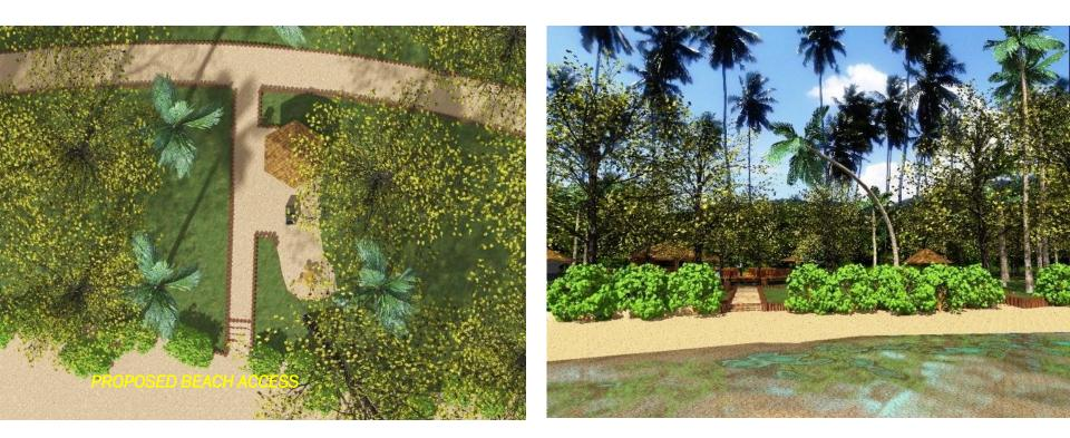
Access to the beach for the park users will be restricted to the designated accesses from the footpaths of the interior of the park. Such accesses will be of the same design as of the interior footpath only smaller. At the end of each access will be a series of timber based steps similar to the ones implemented at Anse a La Mouche. Eroded parts of the sand dunes will also be stabilized with the same features.
